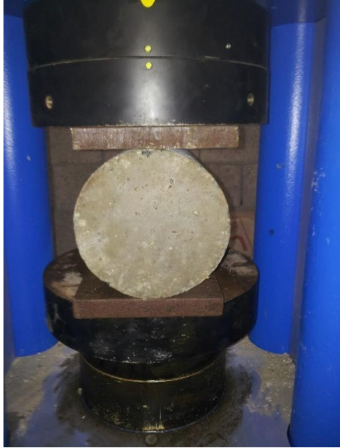
Figure 3.16: Split cylinder test
