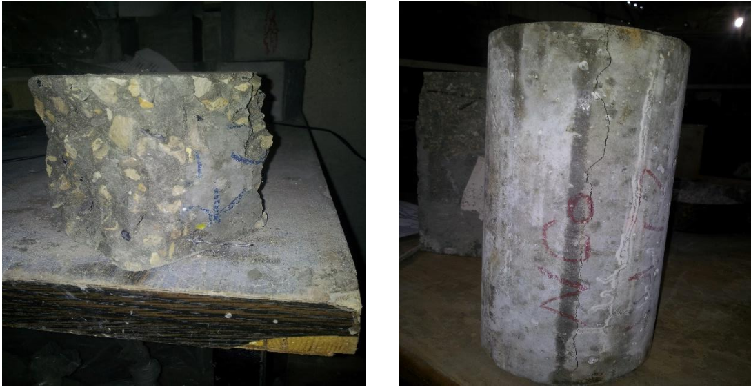
Figure (7) Failure Mode
