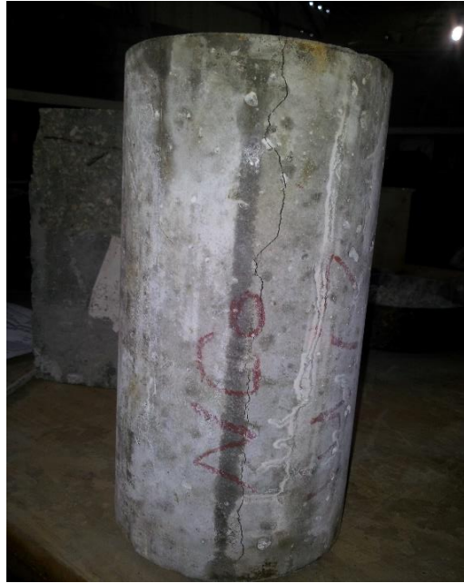
Figure 3.17: Cylinders damages after test
