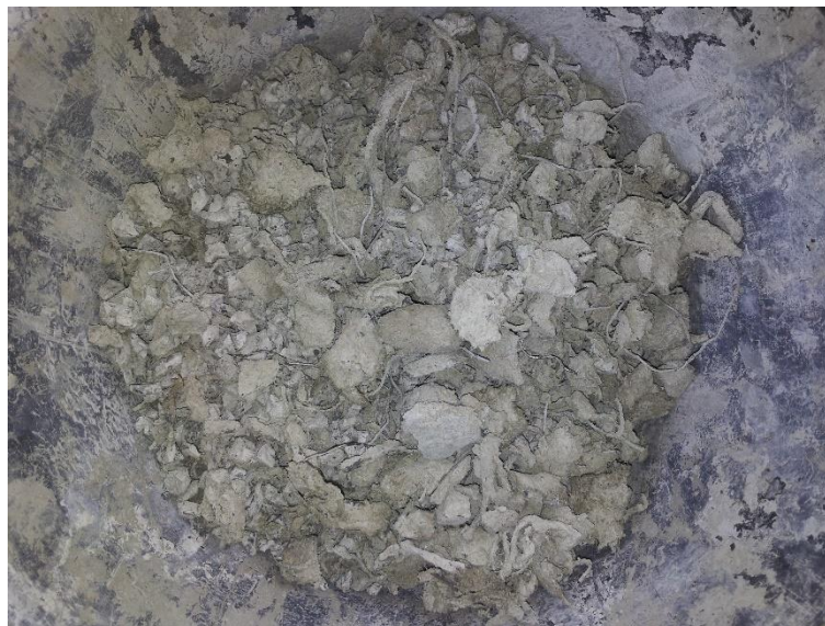
Figure 3.12: Rubber aggregates after mortar pre-treating
