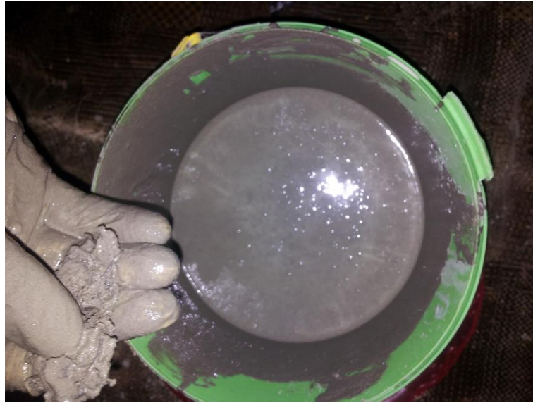
Figure 3.13: Rubber aggregates with mortar by adding bonding agent pre-treating
